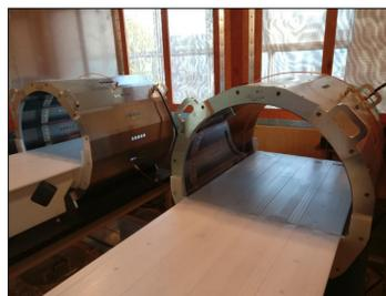
Figure 1: MITS 1.5/64 MHz (left) and 3.0/128 MHz (right) bench top exposure systems [3].
